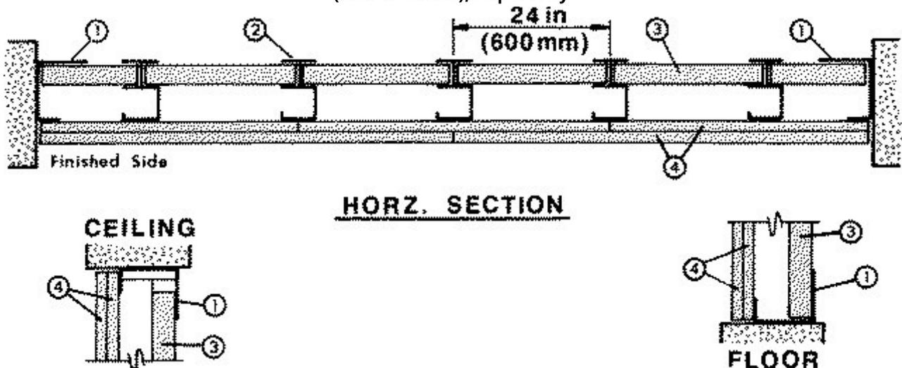
1. **Floor and Ceiling Runners** — "J" -shaped runner, 2-1/2 in. wide with unequal legs of 1 in. and 2 in., fabricated from 24 MSG galv steel (min 20 MSG when Item 4B is used). Runners positioned with short leg toward finished side of wall. Runners attached to structural supports with steel fasteners located not greater than 2 in. from ends and not greater than 24 in. OC.
