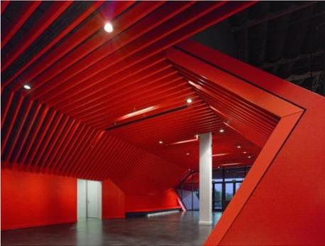
**Description:** Barz™ is a linear ceiling system consisting of precision, factory detailed panels attached to a concealed carrier suspended from the structure above. A variety of perimeter and transition details are available with the Barz™ system. Torsion spring attachment of cassette allows for easy access.
