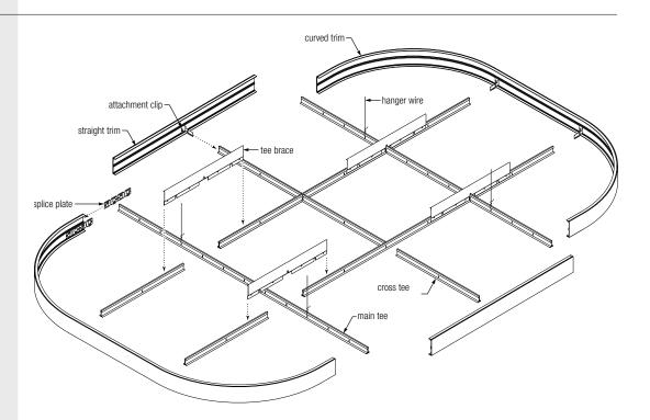
Panels not included. Thorough component and full scale load tests were conducted to ensure performance with a variety of infill panels and loading conditions. Infill panel weight shall not exceed 4lbs. (1.81kg.). Solid wood panels are not recommended.
