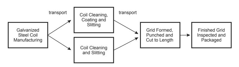
During the grid production process, a piece of galvanized steel coil (destined to be the body) and a second piece of coated galvanized steel coil (destined to be the cap) are combined into the proper configuration using a series of driven dies. A clip is attached to both ends of the main tee and cross tee members allowing for connection of the various pieces.
