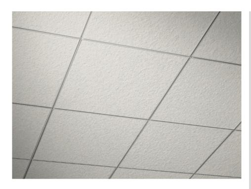
Offering a monolithic ceiling look with every benefit of an economical grid system. USG Donn® Brand Fineline® DXF™/DXLF™ Acoustical Suspension System allows for easy ceiling access, while its narrow slotted profile, with a 9/16" wide face and a 1/4" reveal, hides the suspension system behind acoustical panels. Its 1/4" slot accommodates partition attachments and pendent mounted light fixtures.
