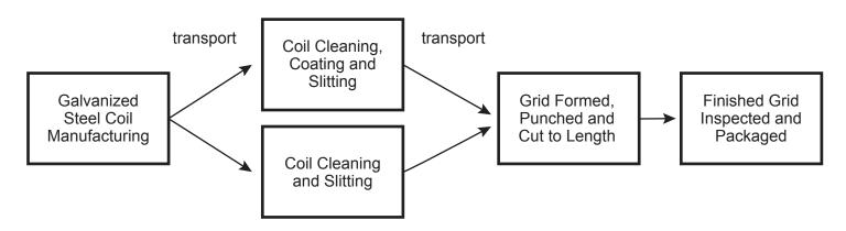
During the grid production process, a piece of galvanized steel coil (destined to be the body) and a second piece of coated galvanized steel coil (destined to be the cap) are combined into the proper configuration using a series of driven roll forms. A clip is attached to both ends of the main tee and cross tee members allowing for connection of the various pieces.
