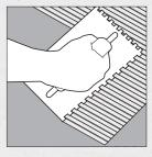
Working a small area at a time, press tile into place with a slight twisting motion to seat properly. Prevent adhesive buildup on tile edge and in grout space. If adhesive squeezes from under tile, remove excess before it dries.
