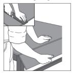
To make cutouts for pipes and fixtures, use a utility knife to cut through facers on both sides and remove foam core. Or, use an electric drill with a hole-saw bit.
