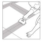
Fill joints with latex-fortified mortar or Type 1 organic adhesive and immediately embed USG Durock™ Brand Tile Backer Tape or equivalent alkali-resistant, fiberglass mesh joint tape.
