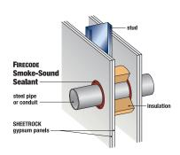
FIRECODE Smoke-Sound Sealant is classified for use in through-penetration fire stop systems C-AJ-1020 and W-L-1064 and complies with IBC requirements for smoke barriers.
