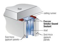
A UL-classified fire and smoke caulk, FIRECODE Smoke-Sound Sealant is ideal for head-of-wall and bottom-of-wall systems in fire-rated partitions and smoke barriers.
