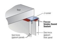
FIRECODE Smoke-Sound Sealant is also rated for joints in shaft wall assemblies and can be used with most liner panel systems, including, but not limited to, U415.
