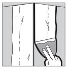
6 Use an 8" or larger finishing knife for outside corners (4"-6" knife for inside corners) to apply a finishing coat of compound. (Do not use DURABOND or taping joint compound for this step.) Feather compound 8" (200 mm) from nose of trim for outside corners (1" (25 mm) past previous coat for inside corners). Let dry; sand and prime.
