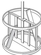
the mix. Operated at proper speed, the paddle mixes thoroughly, producing a virtually air-free plaster.
