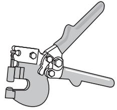
**Pop Rivet Tool** Plier-type tool used to flare and secure pop rivets through prepared holes. Especially useful for securing wall angle corners or tee joints in suspended acoustical ceiling applications.
