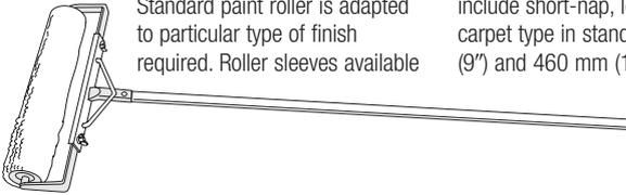
Standard paint roller is adapted to particular type of finish required. Roller sleeves available
