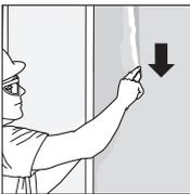
Creased THERMAFIBER application—THERMAFIBER SAFB 25 mm (1") wider than stud cavity is field cut with utility, carpet or hook-blade knife. Crease will press against gypsum panel to dampen sound vibrations.
