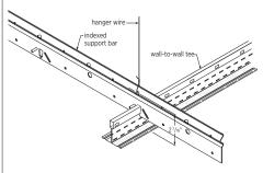
Main tees must be supported at both ends when hanger wires are used
