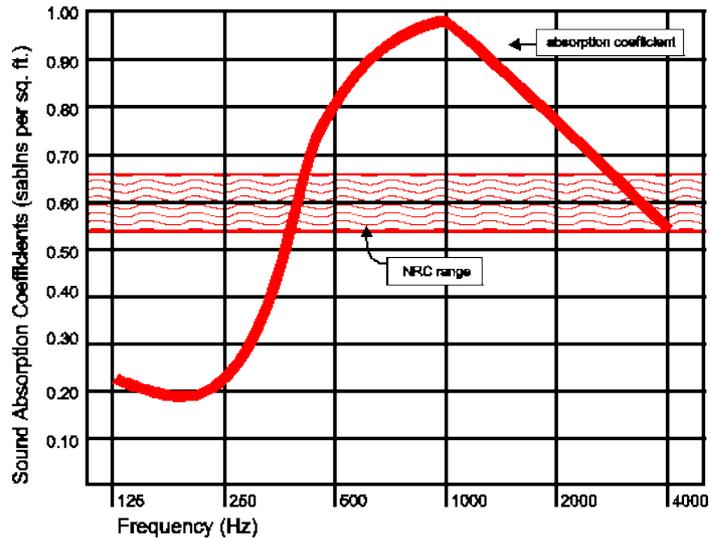
As shown in Figure 14 (above), an acoustical product which absorbs sound will at one frequency may be very inefficient at other frequencies. In short, absorption coefficients represent maximum performance at each frequency while an NRC value represents an average of the absorption at four frequencies.
