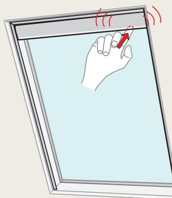
**ENGLISH:** Turn on the power to the shade by pressing the power switch at the bottom of the shade for one second.
