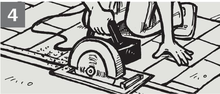
Cut the roof opening as marked and remove the roof decking. If an intermediate roof rafter is to be cut, it may be necessary to temporarily support it until a header can be installed. NOTE: Using a circular saw, make a slot cut 1½" back from the opening and above the rafter to be cut. This will allow you to cut the rafter with a handsaw and leave space for the header.
