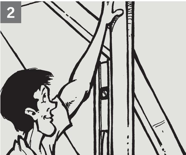
Locate the two bottom corners of the skylight opening on the underside of the roof deck, relative to the ceiling opening and type of well. Mark these points on the roof by driving nails through the roof deck. Measure up from the two nails the appropriate distance as required by your unit (refer to chart below) to locate the top corners of the roof opening and mark them with nails also.
