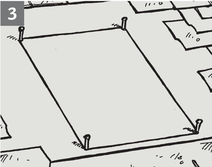
Move to the roof and using the four nails as guides, remove the shingles (but not the felt paper) to approximately 12" back from the top and sides of the roof opening (as shown by the nails) but only 2" back from the bottom edge.
