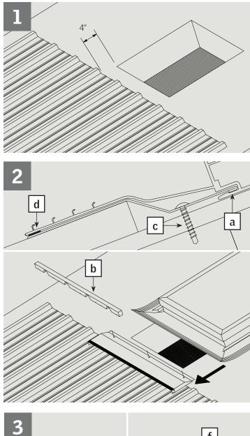
Install roofing to 4" from the bottom edge of the skylight rough opening. Grind or file any sharp edges on the roof panel that are less than 8" from the opening.
