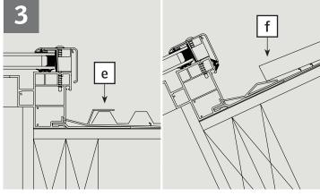
Install roofing around the unit sides under the water diverter gasket (**e**), and over the water diverter gasket at the top ( $\mathbf{f}$ ).
