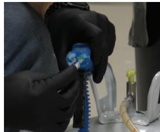
Application of petroleum jelly to spray gun
