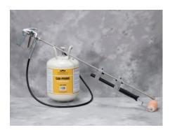
Versico's V-150 Primer packaged in a pressurized cylinder for spray application. V-150 Primer is a solvent-based product designed for one-step cleaning and priming of EPDM surfaces prior to the application of quick-applied (QA) products. CAV-PRIME primers are applied using a self-contained spray system coupled with a spray aun with extension wand and applicator attachment kit. CAV-PRIME spray guns, hoses, and applicator attachment kits are sold separately.
