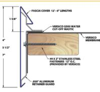
Available for Fully Adhered and Mechanically Attached Systems (shown) Ballasted version also available.
