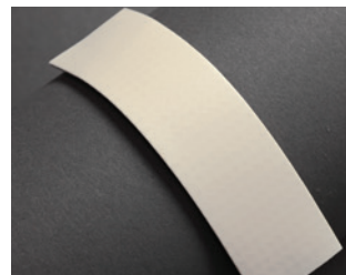
Versico VersiWeld – 60 Weeks (No Failure)
