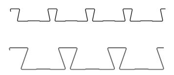
The Vulcraft Structural DoveTail Ceiling/Deck is available in 2-inch-deep and 3.5-inch-deep profiles.
