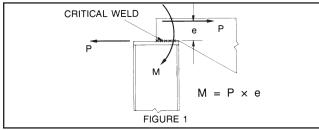
Vulcraft has done extensive testing of the maximum eccentric top chord force capacity for joist girders. Based on this test program, the maximum horizontal load for 7.5 inch deep seats are presented in Table 1 (below)
