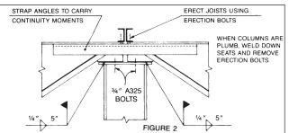
When the end moments on the Joist Girders are too large for the seat to resist, it is necessary to utilize a moment plate as shown in Details A-F. The use of this simple moment plate virtually eliminates all eccentricity problems.
