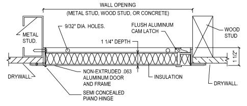
This lightweight, insulated, all aluminum access door is ideal for exterior applications, and also those specific interior applications where corrosion or moisture is a concern. Access to large openings in walls and ceilings is made easy. The non-extruded door frame has the same visual aesthetic design as the GP 100 Series door. Comes with gasket on 3 sides. The aluminum door panel is insulated with 1" TUFF-RTM polyisocyanurate.
