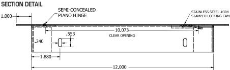
This lightweight, insulated, all aluminum access door is ideal for exterior applications, and also those specific interior applications where corrosion or moisture is a concern. Access to large openings in walls and ceilings is made easy. The non-extruded door frame has the same visual aesthetic design as the UAD Series door. Comes with gasket on 3 sides. The aluminum door panel is insulated with 1" KINGSPAN GreenGuard Insulation.
