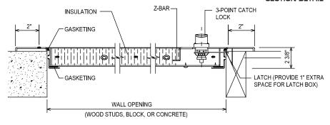
The one of a kind exterior access door is galvannealed \* \* steel, insulated with 1" GreenGuard and includes double seal gasketing. Weather resistive gasket on inside for outdoor applications (certain saltwater areas might not be compatible).
