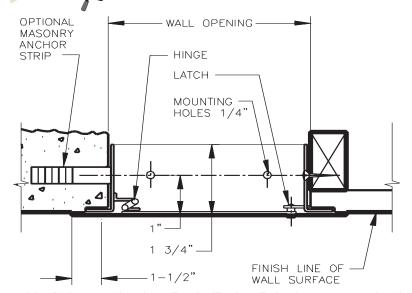
This precision-flush access door for wall and ceiling installation far surpasses other doors. Laser cut, no corner mitering – aesthetically preferred by architects and building professionals.
