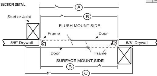
The MAP 1800 plastic access door is high impact ABS plastic reversible panels with UV stabilizers made with precision dies for perfect fit of door and frame. Surface is a cosmetically acceptable textured surface.
