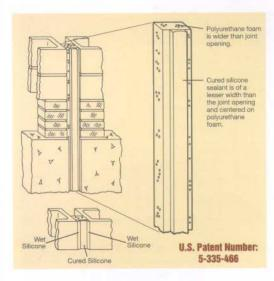
**Description:** Everlastic Wide Joint Seal is a factory cured strip of silicone sealant adhered to rectangular polyurethane backer. The polyurethane backer is wider than the joint opening.
