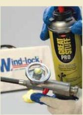
**4.** After removing the can from gun, clean the gun adapter with the Dow\* Cleaner.
