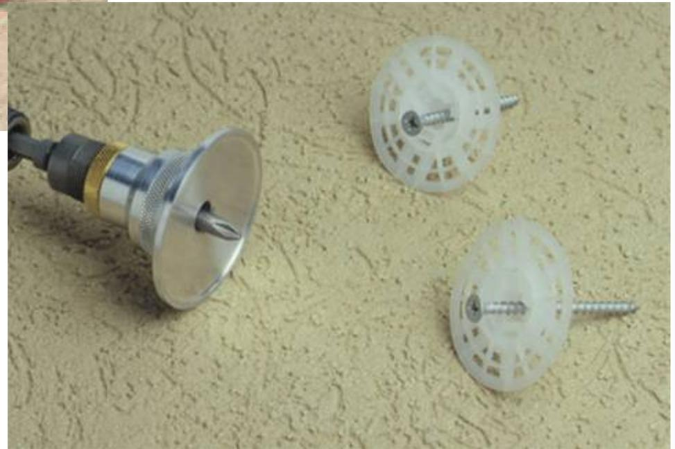
**Note:** For proper and consistent installation of mechanical fasteners, utilize a depth stop attachment on your screw gun.
