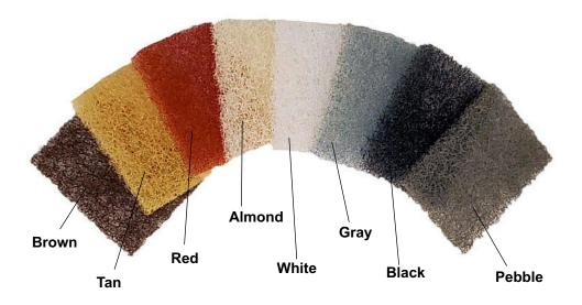
Mortar Net® Weep Vents™ are made from recycled polyester with a 90% open mesh, and are bonded with a flame retardant adhesive to provide resiliency and strength, plus an anti-microbial additive to control mold growth. They are an easy way to ensure brick cavity and single wythe block construction masonry walls maintain their finished appearance and drain correctly for life.
