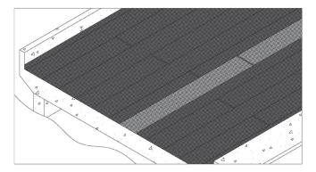
tack coat must be applied to the membrane surface prior to the placement of the asphalt overlay. The reason for this tack coat is to address potential concern with decreased asphalt content in overlays that is essential for good adhesion to the membrane. In the event of rain, the membrane surface must be dried prior to asphalt placement.
