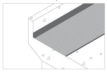
sheets from low point to high point in both the longitudinal and transverse directions. On flat deck surfaces, start at one curb and proceed across to the other. Measure the width of the deck (in feet) in at least three places and divide the widest number by three feet (the width of a sheet minus the overlap) to get the number of sheets it will take to cover the deck width.
