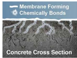
When used on fresh concrete, PENCURE OTC cures the concrete and performs similar to a post 28-day penetrating sealing compound application, offering less down time and reduced installation cost compared to what multiple coats require.
