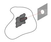
Cut a piece of DETAIL FABRIC to the dimensions of the soil nail plate and embed the fabric into the previously applied HYDRALASTIC 836.
