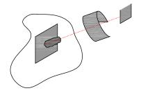
**5.** Cut another two pieces of DETAIL FABRIC, one for the shaft of the soil nail, the other for the top, and embed this fabric into the previously applied HYDRALASTIC 836.
