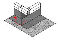
4. Install overlapping PRECON according to installation instructions onto soil stabilization system. Cut PRECON on the horizontal to allow for ease of bending around corner.
