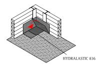
**4.** Apply HYDRALASTIC 836 to the area of PRECON that will be accepting the PRECON overlap, fold down overlap and embed in the HYDRALASTIC 836. Roll press into place.
