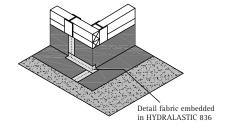
6. Apply HYDRALASTIC 836 at all overlapping joints in a 12" wide application and then fully embed detail fabric into this HYDRALASTIC 836. Terminate all edges with additional HYDRALASTIC 836.
