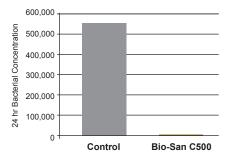
Concrete was cast in  $100 \times 200$  mm cylinders with both control and treated mixes. A wastewater facility was chosen that had elevated  $H_2S$  levels and substantial existing MIC corrosion damage. Test samples were suspended in the air space of the tank for 10 years. Exposure trials showed that treated concrete had nine times less concrete mass loss compared to control samples.
