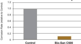
After 10 years, the concrete treated with Xypex Bio-San C500 had 9 times less corrosion than the untreated concrete, and continued to function at full efficacy.
