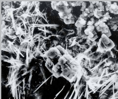
XYPEX CRYSTALLIZATION (INITIATION)
