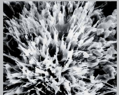
XYPEX CRYSTALLIZATION (MATURE)
