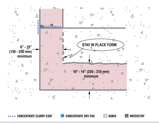
STEP 1: Install stay in place forming assembly as shown to create a shell of Xypex Admix treated concrete around the entire outside area of the matt slab. The shell thickness is to be a minimum of 6" (150 mm) to 10" (250 mm).
