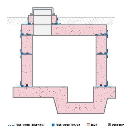
**STEP 1:** Clean joint thoroughly. Between pours apply Xypex Concentrate slurry to joint surface at the rate of 2.0 lb./sq.yd. (1.0 kg/m²).
