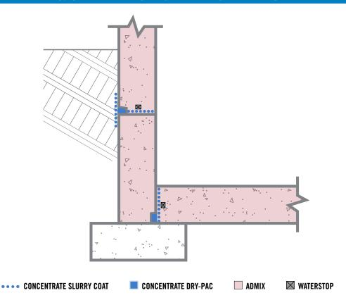
STEP 1: Where the slab will contact the wall modify the forms to create a linear groove in the finished concrete surface of the wall. The linear groove is to be aligned with the bottom of the slab and is to be 1½" (37 mm) high by 1" (25 mm) deep.
