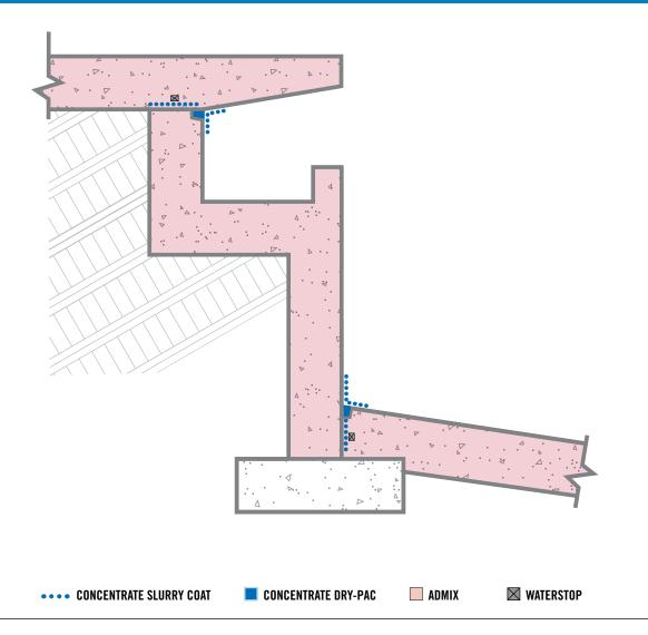
**STEP 1:** Clean joint thoroughly. Between pours apply Xypex Concentrate slurry to joint surface at the rate of 2.0 lb./sq.yd. (1.0 kg/m²).
